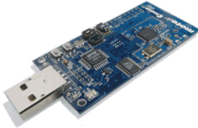
Figura C.1: Dispositivo Tmote Sky - IEEE 802.15.4 compliant device for wireless mesh networking featuring a 250kbps radio, 10kB RAM, 48kB flash, and 1MB storage
